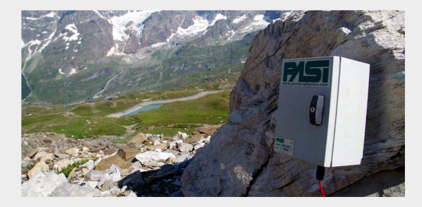
Data from **3C-land geophones** (2Hz) are acquired by the 4-channel, 24 bit data acquisition board and automatically saved on the internal SD memory; the timing of the internal GPS allows the synchronizations of more GeaGPS units even if they are not physically connected together. This leaves the researchers free to choose the best location to mount each single station in the field, as any of them will be able to operate in total autonomy.
