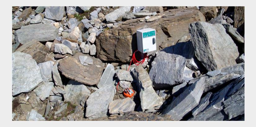
In order to acquire seismic data for a long time in remote areas characterized by extreme temperature excursions and severe meteorological conditions (like the Italian Alps), GeaGPS was designed with internal batteries to warrant at least 1 month operations; the use of a solar panel can obviously extend the autonomy of the battery itself.
