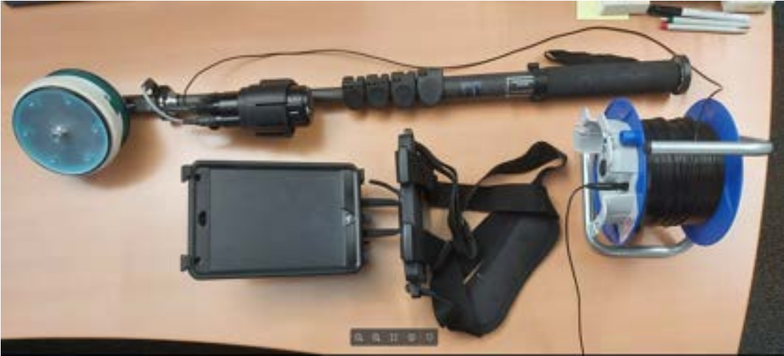
Figure 8 : PM8500 One wheel electrode cabling set up
