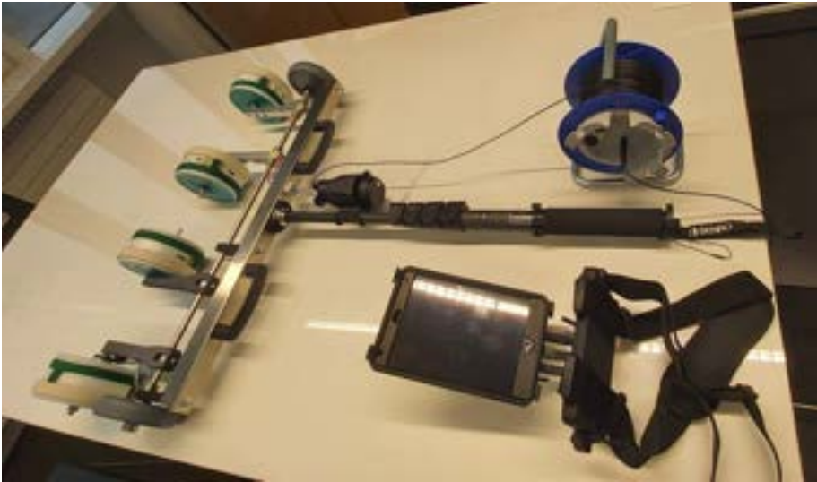
Figure 9 : PM8500 Four-wheel electrode cabling set up
