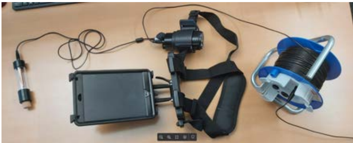
Figure 7 : PM8500 Rod electrode cabling set up
