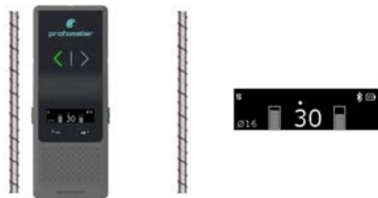
Figure 47: Approaching a rebar with signal strength indicator
