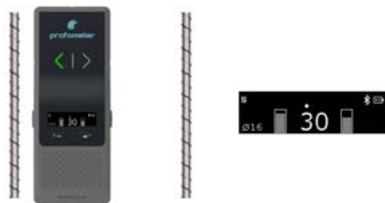
Figure 47: Approaching a rebar with signal strength indicator
