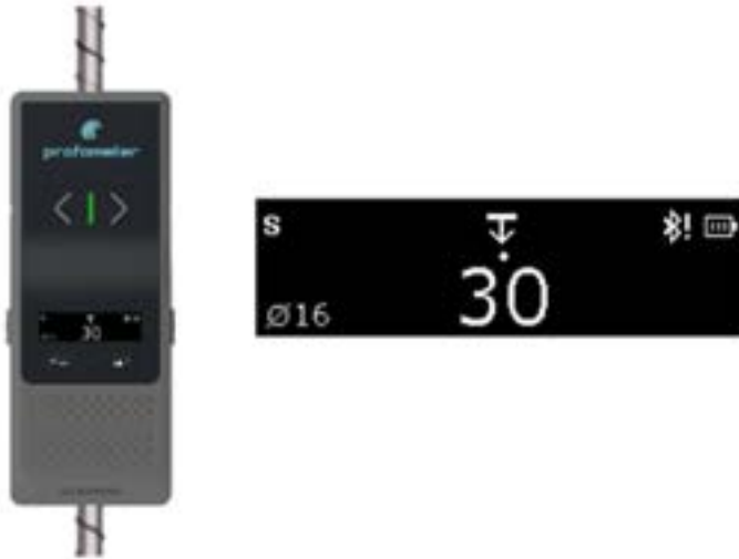
Figure 40: Indication of a rebar
